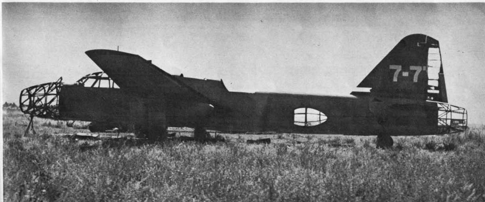
PEGGY Army bomber carries either torpedoes or bombs, may even take part in Kamikaze suicide attacks. Top speed is nearly 350 m.p.h. Recognitionally Peggy is a cross between Helen
